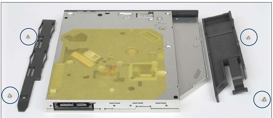
Figure 133: Replacing the optical drive in the installation frame
